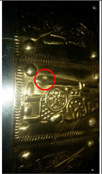
*Depression in brass caused by finger nail, indicating material is quite soft and consequently not ideal as a joining material*
