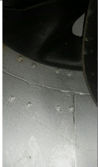
*Photo of other side, faintest of spot welds present showing attachment of kicker to dome.*
